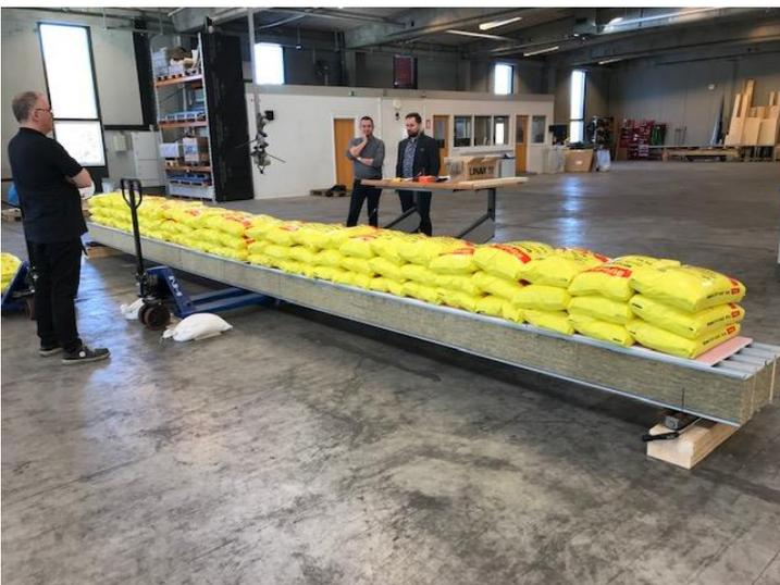
Loading with 9 sacks per meter beam
