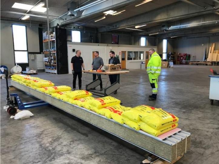
Loading with 5 sacks per meter beam
