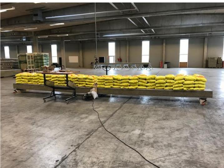
Loading with 12 sacks per meter beam
