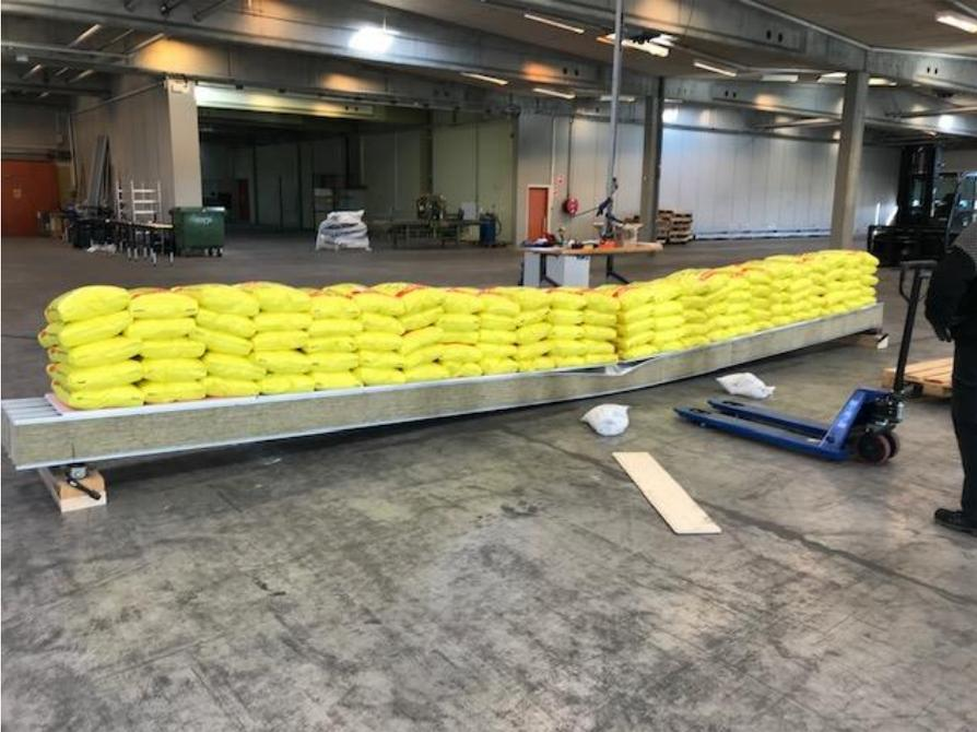
Loading with 15 sacks per meter beam – failure - folding of top flange
