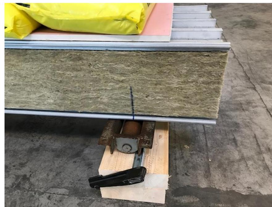
Deflection measuring equipment, located in the mid section of the beam/element.
