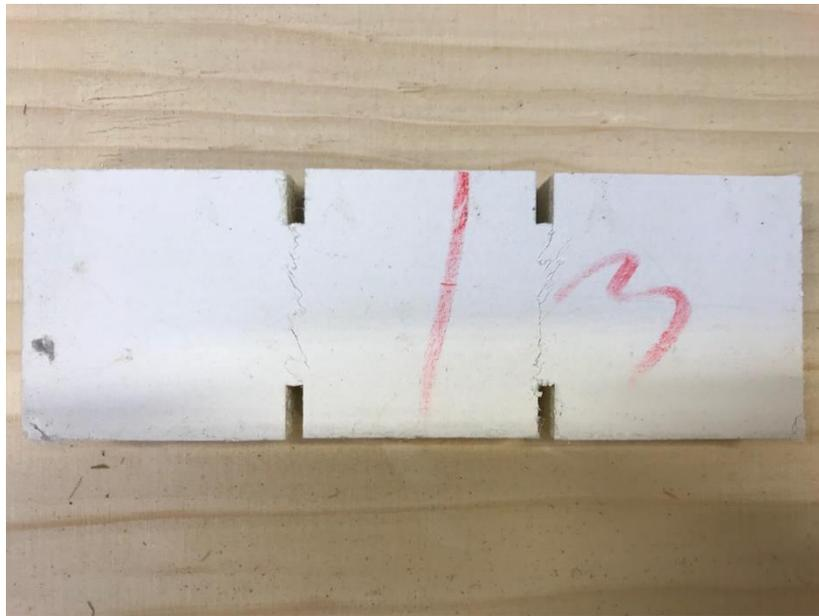
Typical failure modes - "para" test specimens
