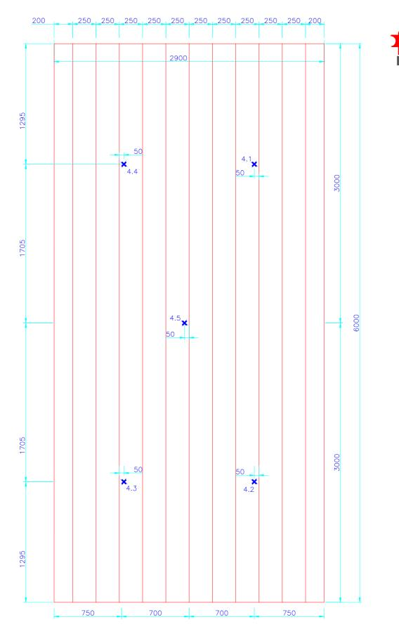
★ Thermocouple placed on exposed side of the test specimen between the test specimen and the 2x15 mm gypsum boards
